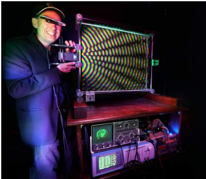
Fig. 5. Photograph of the interference patterns between the capacity to sense of a matched pair of Shure SM58 microphones. The SWIM apparatus (e.g. lock-in amplifier, etc.) is also visible in the picture. Figure reproduced from[2].
