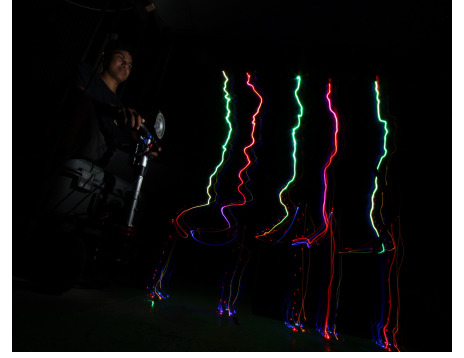
Fig. 11. Multi-exposure photo of drone using PID controller to fly path of constant phase. Horizontal flight path constantly adjusted to find desired phase. Green represents 180^\circ phase, red 0^\circ .
